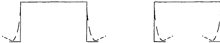
Fig. 3.3 Distortional mode controlled by simple lips
